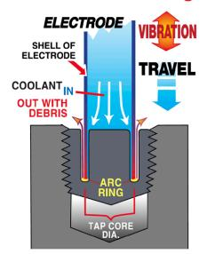
To work well, the length and intensity of stroke (vibration) and the arc voltage must be precisely co-ordinated. Electro Arc disintegrator heads and power supplies are built to provide that precision, with factory settings optimized for maximum performance.
