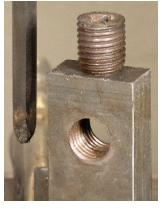
Carbon electrodes can come in different cross-sections like the square electrode shown. It made a square hole in the bolt so it could be backed out with a wrench.
