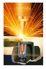
material away between arc cycles. That's done by high-pressure coolant flowing through the tubular electrode. Flushing out happens as the electrode is pull back on each upstroke.
