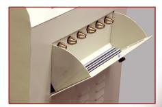
Convenient tool storage drawer with six collet holders and space for electrodes
